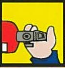
Aim low, pointing the extinguisher nozzle (or its horn or hose) at the base of the fire.
