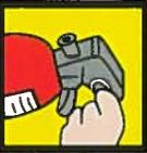
Pull the pin. Some extinguishers require unlocking a latch, pressing a puncture lever, or other such motion.
